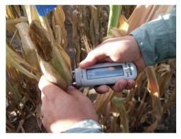
Figure 2. Measuring grain moisture with Voltcraft FM-200 Humidity meter, trough the husks
