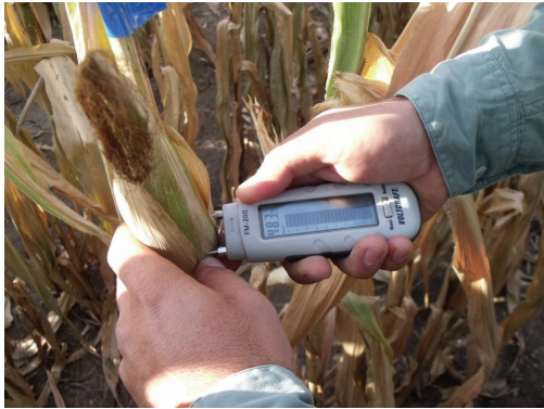
Figure 2. Measuring grain moisture with Voltcraft FM-200 Humidity meter, trough the husks
