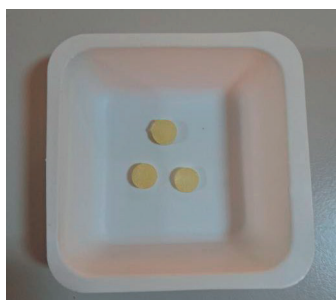
Figure 1. Hydrogel samples obtained through electron beam radiation
