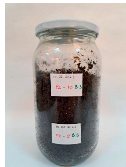
Figure 2. The biodegradability system which includes two hydrogel samples
