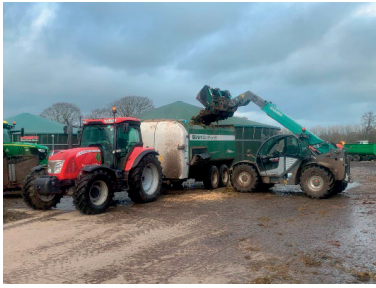
Figure 1. Trailed feeder wagon with the associated tractor and telescopic handler unit
