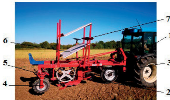
Figure 1. Machine for planting vegetable seedlings and medicinal plants in a row, MPA symbol (INMA, 2018)
