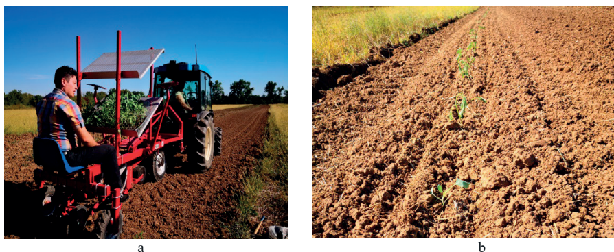
Figure 2. MPA: a- seedling planting machine during experiments; b- planted seedling
