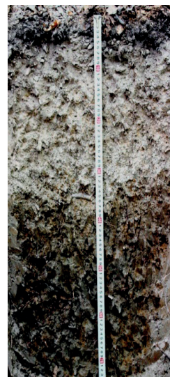
Figure 2. Profile 12. Greyzem albic, stagnic slitized, gleyzed from the surface, clayey-loamy 0-37 cm, loamy-clayey 37-80 cm, strongly differentiated textural (altitude 249 m, hornbeam forest, Rezina)
