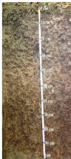
Figure 1. Profile 11. Greyzem typical, moderately humic with semi-deep humiferous profile, semi-deep clayey-loamy, moderate differentiated textural, virgin (altitude 258 m, oak and carpen forest, Briceni)
