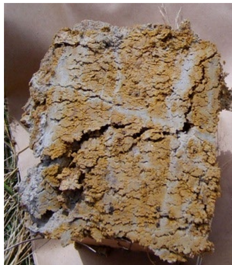
Figure 8. Bt 2 W horizon (88-108 cm): at morphological level (in the soil profile) the greenish-gray network is very well expressed (with clear angles of 90°)
