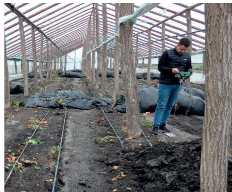
Figure 2 Determination of penetration resistance in Pahnesti plastic tunnel
