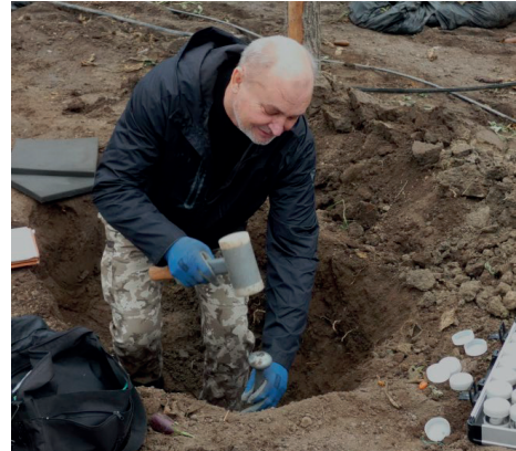
Figure 1. Sampling of soil in stainless steel cylinders to assess the state of soil compactness - three replicates
