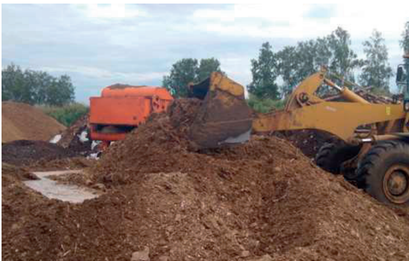
Photo 2. Mixing of volumes of introduced mushroom production wastes using mechanization mean
