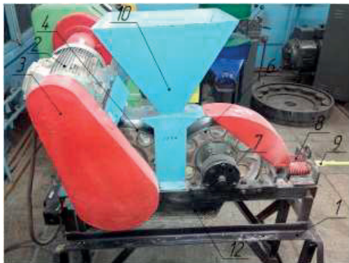
Figure 1 - Design and general view of the roller conditioner (Petent, 2008): 1 - frame; 2 - electric motor; 3 - V-belt transmission; 4 - drive roll; 5, 7 - bearing support; 6 - driven drum; 8 - safety spring; 9 - adjustment screw; 10 - loading hopper; 11 - damper; 12 - unloading tray
