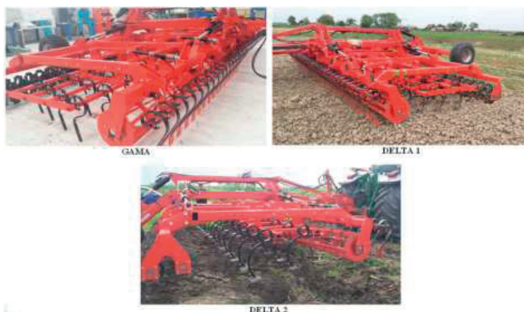
Figure 3. The prototype vibro-combinator SANDOKAN 2 equipped with the three types of active elements (GAMMA, DELTA 1, DELTA 2) (Boja et al., 2018a; Boja et al., 2018b)
