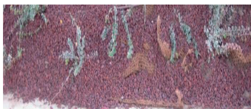
Figure 2. Neds biodegradable jute, expanded clay and vegetation
