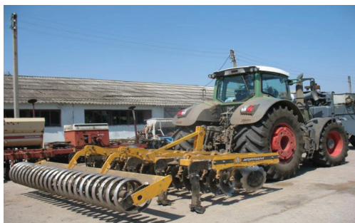
Figure 7. Technique for Implementing the Mini-Till Soil System in Combination with subsoiling to work the land polygon basic of research
