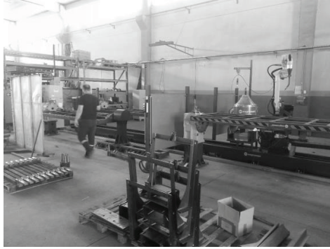
Figure 4. Robot welding used during welding of field sprayer chassis and booms
