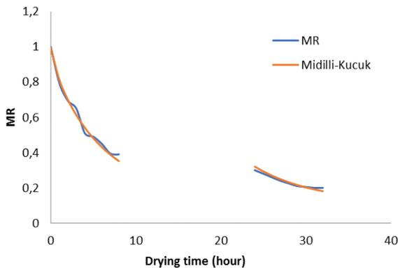
Figure 2. Variation of moisture ratio with drying time for solar tunnel drying of white mulberry
