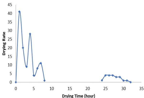
Figure 3. Variation of drying rate as a function of drying time for solar tunnel drying of white mulberry
