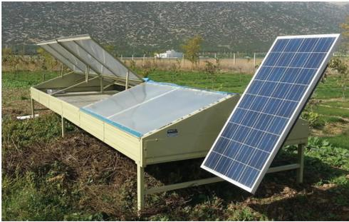
Figure 1. The experimental solar tunnel dryer
