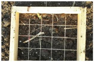
Figure 9. Degree of mixing with circular disk
