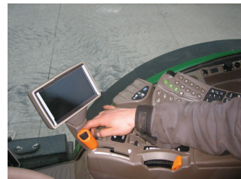
Figure 4. Operator’s right arm position when using a John Deere CommandARM
